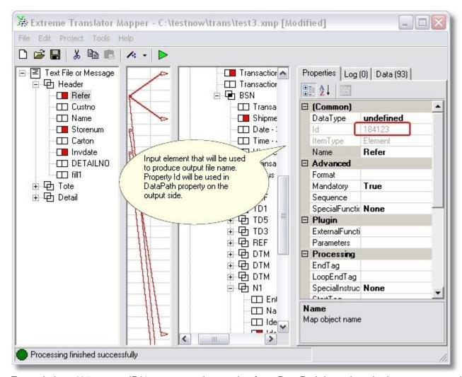
Example how %#propertyID% macro can be used to form DataPath based on the input or output data. See next screen shot for more details.
