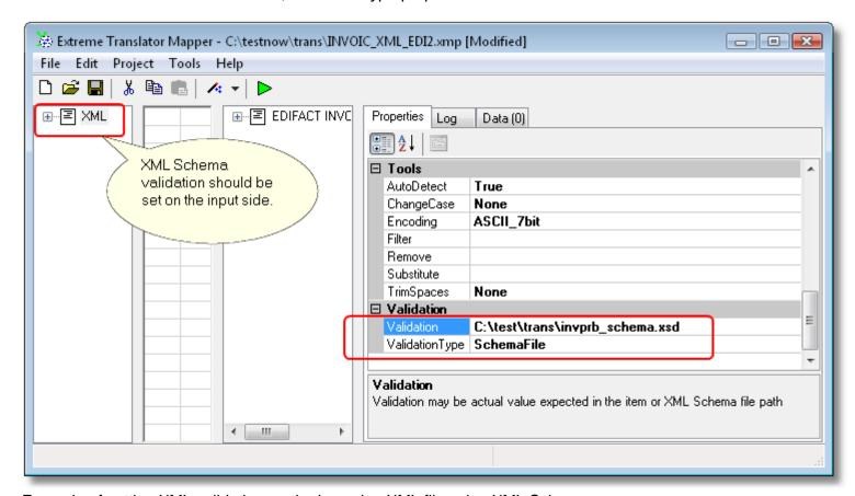
Example of setting XML validation on the incoming XML file using XML Schema.
