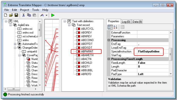
Also to have all the headers line up with details SpecialInstruction property has to be setup to FlatOutputInline on first detail item in the flat file.
