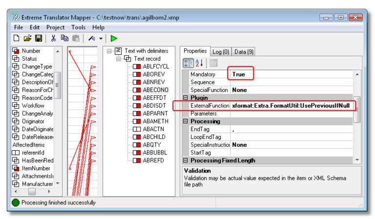
There is example of XML mapping to flat text file with comma delimiters. In this example header data has to repeat per each line of detail, so UsePreviouslfNull plug-in function is used to fill in empty spots.
