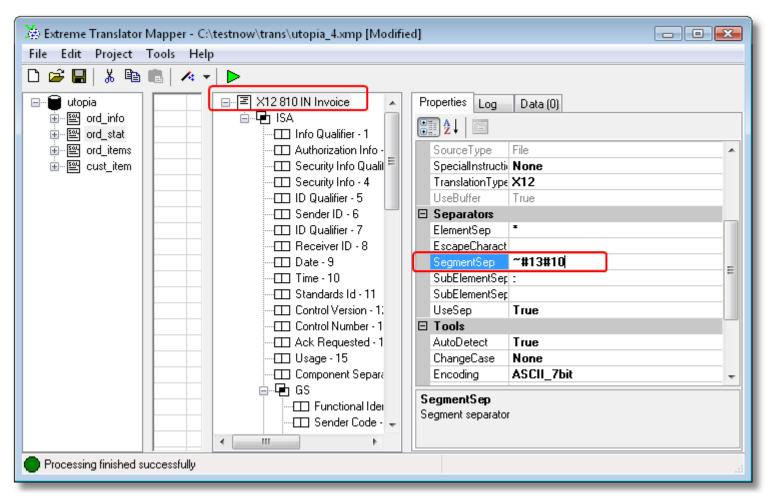
There is how to use non printable characters in properties. In this example carriage return and line feed is placed in the output file.
