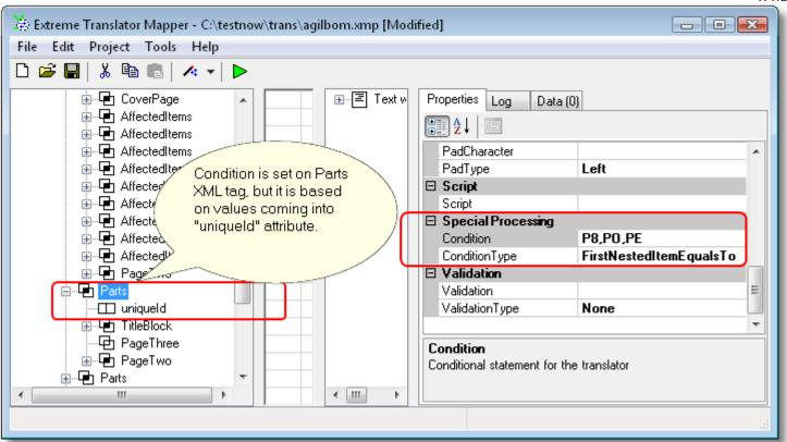
In this example MiscRecord with P8, PO and EQ values is filtered and not placed into the output.
