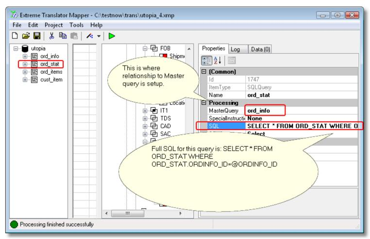
Example of detail query attached to the master. There ord\_info is the MasterQuery while ord\_stat is the detail. For each record of the master, detail is executed and ORDINFO ID is passed into it.
