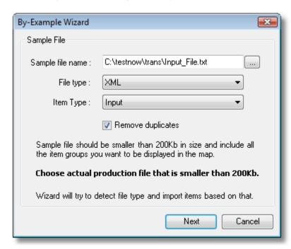
By-Example wizard takes sample file and loads structure into one side of the map.
