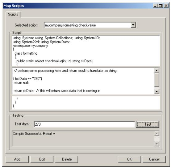
You can use Map Scripts dialog to add and test new scripts. If you click Test button script will be compiled and executed with data from "Test data" edit box assigned to strData variable.
