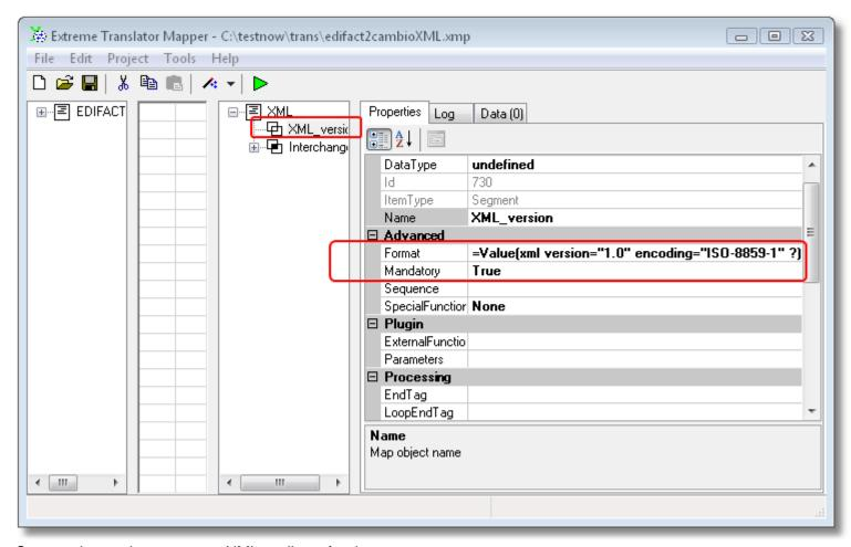
Screen shot on how to setup XML attribute for the output.
